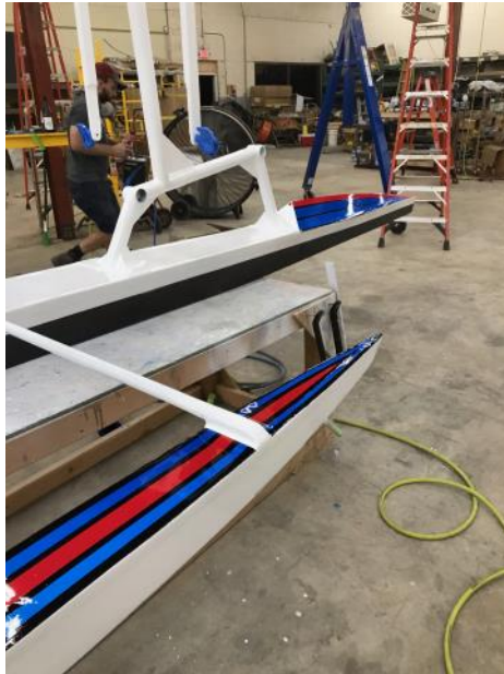
Matt's pedal boat being reconstructed in carbon fiber.
