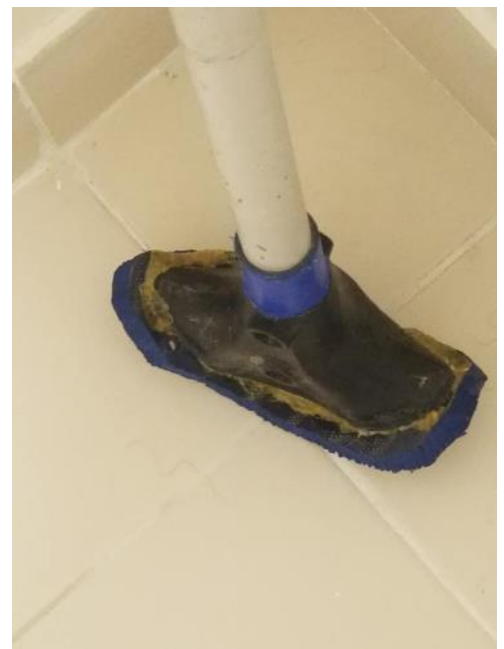
Don's flip-flop land paddle mod. Using contact cement, Don improvised a new grip section when he wore out the stock part and couldn't get a new one easily. He says it works great!
