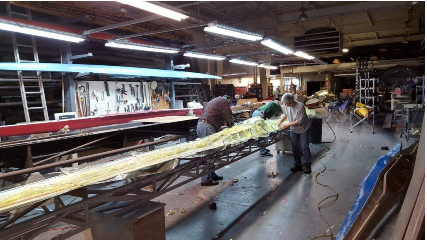
Laying up a new rowing shell inside Van Dusen Racing Boats.
