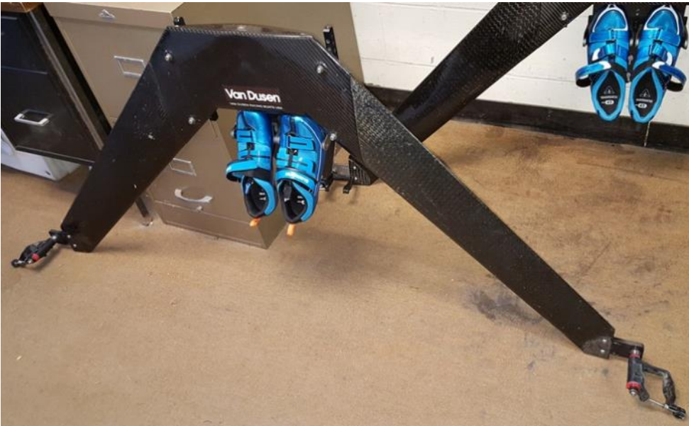
Airfoiled rigger with articulated foot plate utilizing bicycle shoes/cleats.
