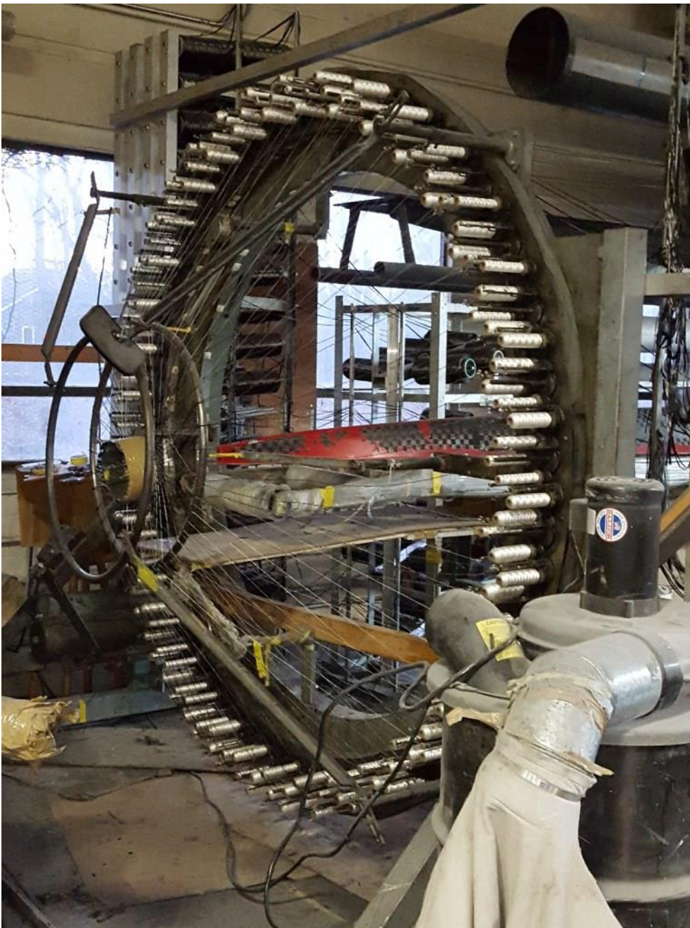
Triaxial carbon fiber yarn braiding machine.
