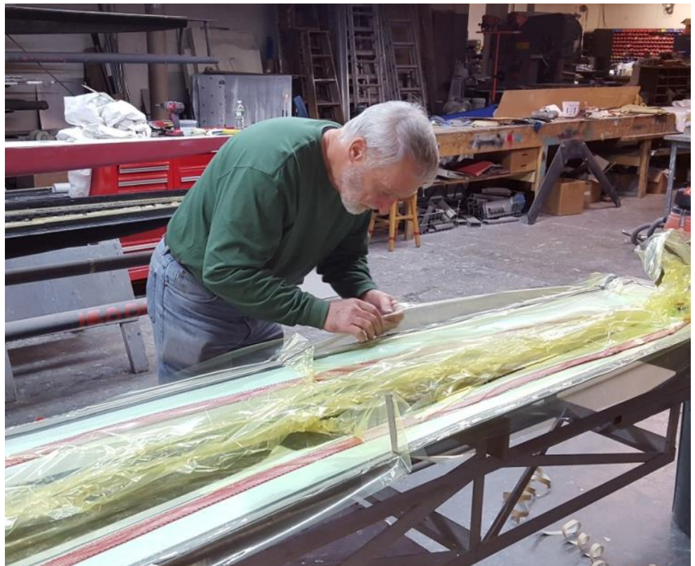
Ted ensuring the vacuum bag has a good seal.
